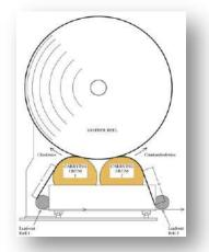
Another important advantage offered by this type of unwinder is that the free paths "A" and "B" (no matter which is the reel rotation direction) are very short and remain the same during all reel unwinding phase.
